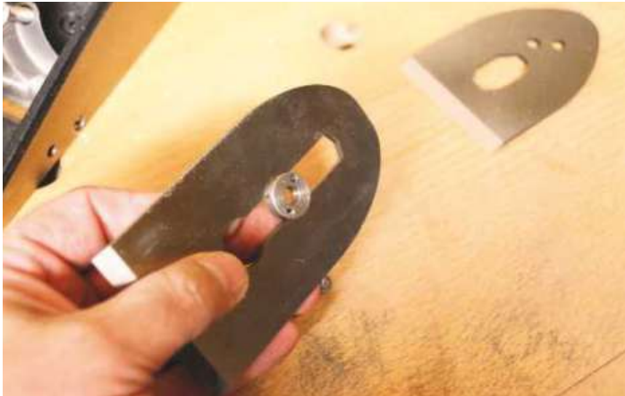
▲ Fully removing the cap screw allows the carrier to stay fixed to the iron for fast resetting
